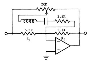
The amplifier summation resistors are equal, and without the filter controls, they give a gain of unity (0 dB). Then if a potentiometer is connected from input to output as shown below, it has no effect on the gain. Next the **RLC** circuit is added. With the pot set at electrical center, the RLC circuit is at a balance position and has no effect on the response. If it is turned all the way to one end, it looks as follows:
