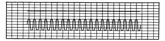
Both curves will measure "flat" on a 1/3 octave analyzer because both have uniform energy in all 1/3 octave bands. But the lower curve (produced by some equalizers) will introduce audible degradation of program material in critical monitoring applications and can trigger acoustic feedback in sound reinforcement installations.
