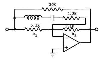
At the resonant frequency  $f_0$  of the LC, the 2.2k resistance is in parallel with the 5.1k, and the gain ratio  $R_2/R_1$  is about 3/1 or +10 dB. Far away from  $f_0$ , the gain returns to unity because L or C is high in impedance and the 2.2k resistance is effectively out of the circuit. Tuning through f gives a band-pass peak in the response that may be adjusted from any value from 10 dB down to flat.
